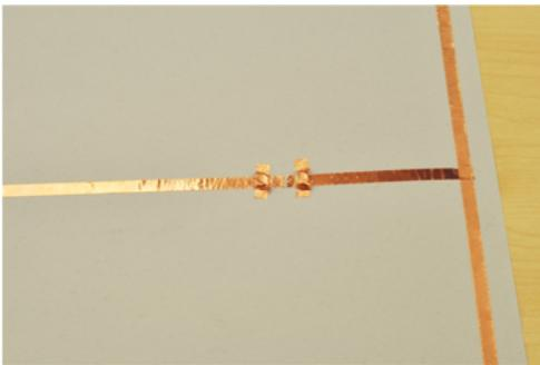
**Figure 3: Fixing magnets on the conductive tape**
