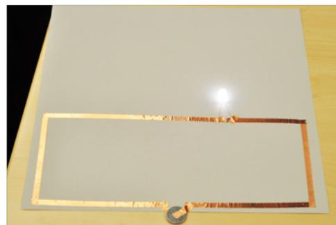
Figure 1: Series circuit with conductive tape
