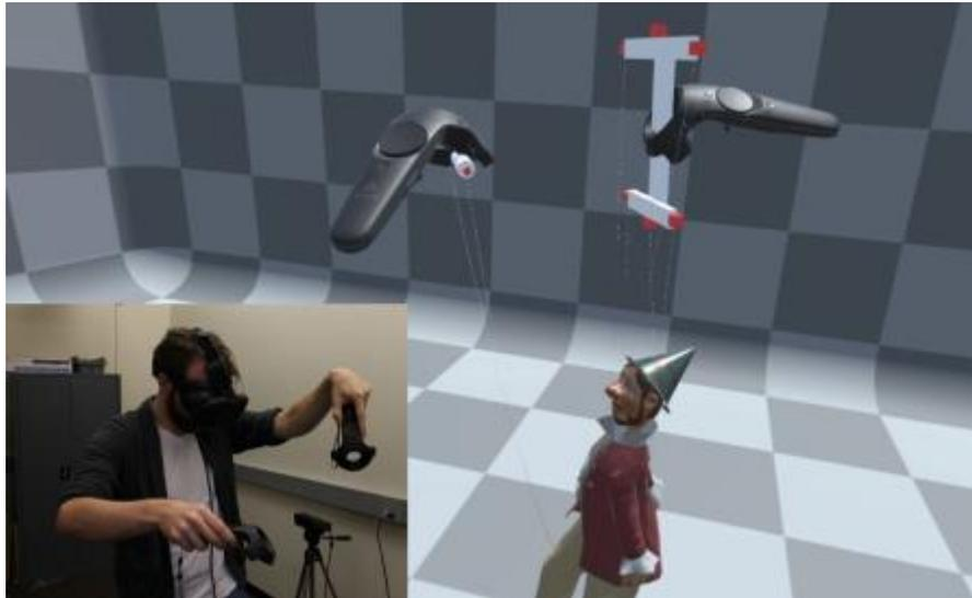
*Figure 2 Prototype in action: Vive system (inlay picture) as it controls a Kasperl body with virtual controllers (larger image)*
